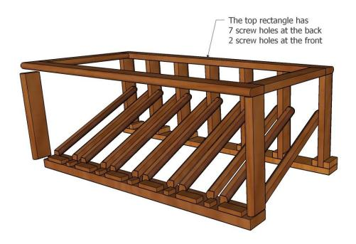
4) Turn the unit upside down and remove the Jig. Screw in the bottom Rectangle into the vertical bars ONLY, 7 screws at back, 2 screws at front.
