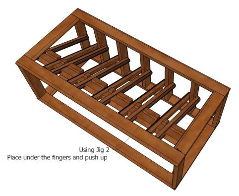
5) Screw in the front finishing bar to complete the 6 bottle display unit.
