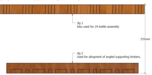
2) Place each of the wine rack Vertical units into the Jig 1, ENSURE that the finger is to the back of the vertical bar and that the cut on the finger is vertical. See image below.
