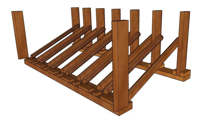
3) Place the open rectangular section on top of the Unit. The TOP rectangle has 7 screw holes at the back and 2 screw holes at the front.
