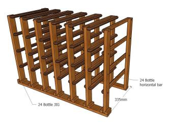
3) Lay the Horizontal bars on top, curve to the front, and screw together.
