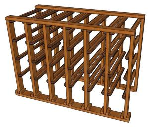
4) Turn the unit upside down and remove the Jig. Screw in the remaining Horizontal bars.
