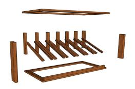
Do NOT use power tools to assemble racking. Hand screwdrivers Only.
