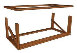
3.) Arrange and screw together Internal supporting bars top and bottom.
