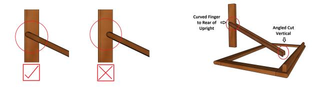
**2.)** Arrange and screw together Front supporting bars, External back supporting bars, Top and Bottom Rectangles.
